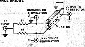
This works on the familiar Wheatstone bridge principle. The unknown impedance is connected to A and the termination (50 ohm dummy lead) plugged into B. The balun uses the Philips balun core 4322-020-3150 or the Neosid 1050/2/R29. For use from about 30 MHz to 200 MHz only a single turn is necessary as shown. For
