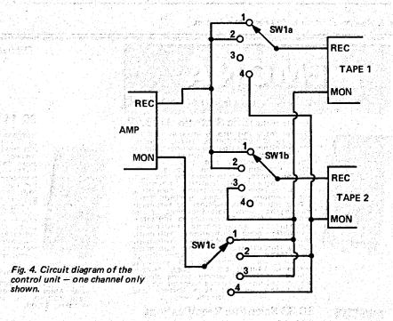
where one three-pole wafer is used for each channel.
