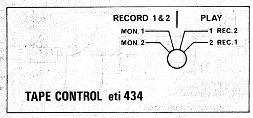
Fig. 5. Front panel artwork. Full size 134 x 58 mm.
