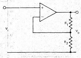
Fig. 1c. Non-inverting amplifier.
