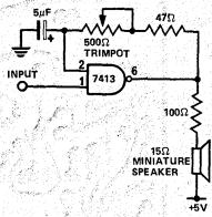
For monitoring slow logic pulses a schmitt trigger is connected as an oscillator. The trimpot controls the pitch of the output. Very useful as a keying monitor or digital clock alarm. When the input goes high, the 7413 will oscillate.
