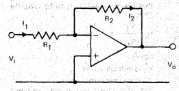
Fig. 1a. Inverting amplifier.
