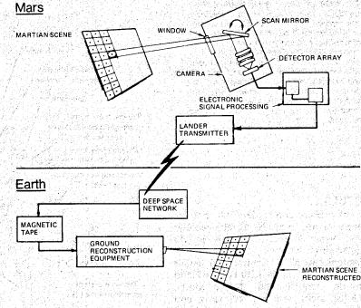
How pictures taken by the television system aboard the Viking Lander will be processed, transmitted and reconstructed on Earth.
