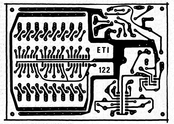
Fig.7. Printed circuitboard artwork. Full size 142 x 104 mm.
