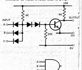
Fig. 3. An early integrated circuit design for a NAND gate in diode-transistor logic — DTL.
