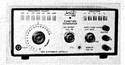
A new high performance, modestly priced function generator (BWD 160) has now been added to the BWD instrument range. The new unit has a frequency coverage from 0.02 Hz to 2 MHz in seven decade ranges, with the selection of 12 different waveforms and five simultaneous outputs. It may also be swept over any four decades by an externally applied log sweep.
