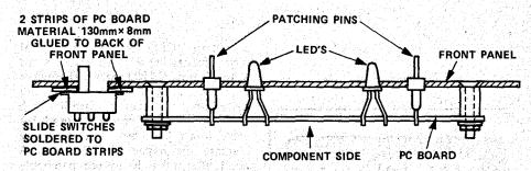
Fig. 5. How the front panel and printed-circuit board are assembled.
