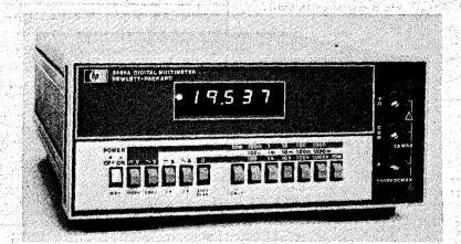
This new 4-½ digit, five-function digital multimeter from Hewlett-Packard combines low cost with high accuracy for both bench and field use. Called the model 3465A, the DMM covers a dc measurement range from 1µV to 1 kV with a mid-range accuracy of ± (0.02% of rdg. + 0.01% of range). AC measure-
