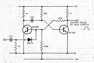
Fig. 17. A basic monostable constructed with discrete components.
