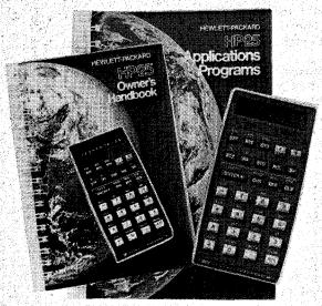
The new HP25 from Hewlett Packard has a 49 step programme with editing and conditional branching, As with all Hewlett Packard calculators very comprehensive owner's and applications manuals are provided with the machine.
