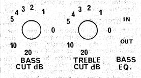
Fig. 3. Artwork for the level control panel. Full size 73 x 50 mm.
