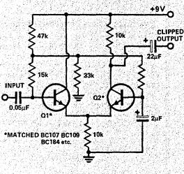
A differential amplifier makes an excellent audio clipper and can provide precise, symmetrical clipping. The above circuit commences clipping at an input of 100 mV. The output commences clipping at ±3 V. Matching Q7 and Q2 is necessary for good symmetrical clipping, however, if some asymmetry can be tolerated this need not be done.
