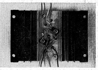
How the completed heatsink assembly appears.
