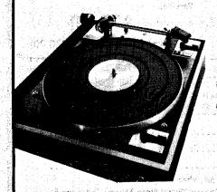
With the CS 601, Dual introduces its second fully auto matic single-play turntable. The CS 601 drive system consists of an 8-pole synchronous motor, developed especially for this new model, and a precision belt running directly from the drive shaft to a flywheel beneath the 305 mm dynamically-balanced platter.
