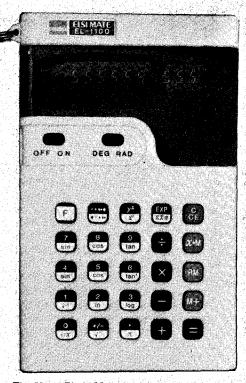
The Sharp EL 1100 has some unusual features. The exponent is displayed in a separate 2-digit display. The key with the unusual notation immediately to the right of the F key converts decimal degrees to degrees, minutes and seconds and vice versa.
