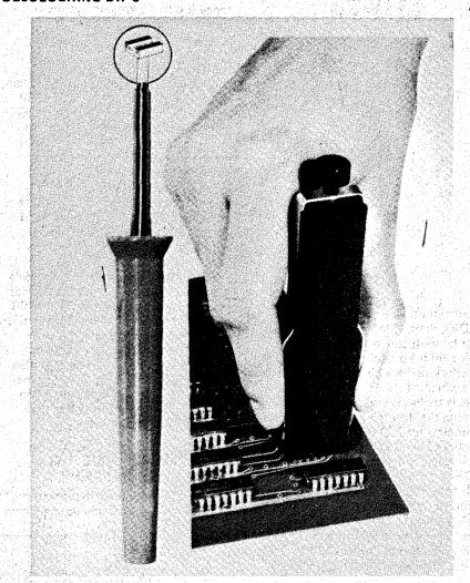
The frustration involved in desoldering and removing dual-in-line packages from printed circuit boards can now be overcome by a 'double-sided' approach suggested by Royston Electronics.
