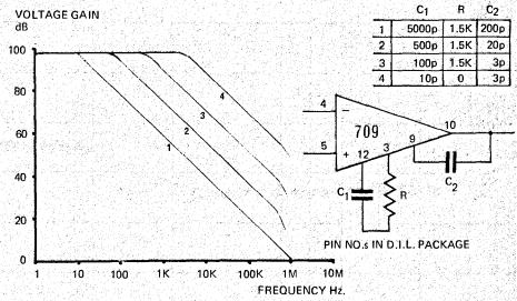
rate of 1 volt/microsecond will limit bandwidth to 10 kHz, if an output swing of 20 volts peak-to-peak or more is required, or to 40 kHz at four volts peak-to-peak.
